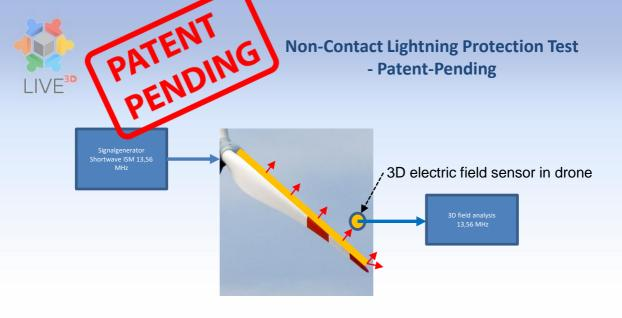
The electic field is always upright to metal. This fact enables the analysis of direction and intensity of the electric field and can prove the existence of an intact earth connection savely.
